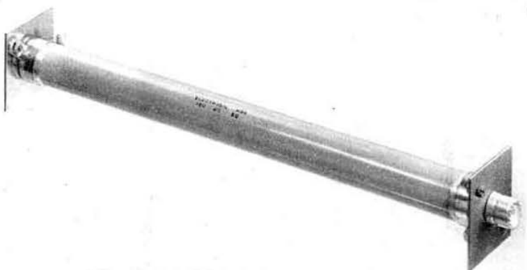
Fig. 1. A 75 ohm Electrosil H39 resistor mounted with 1 in. capacitor clips as a coaxial dummy load.
